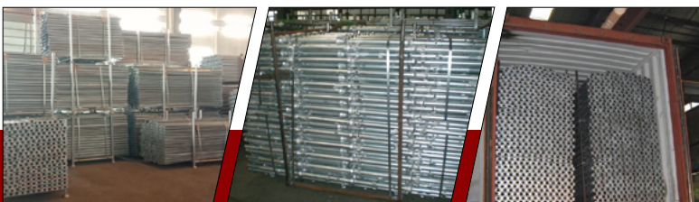
Cuplock scaffolding ledgers in warehouse
