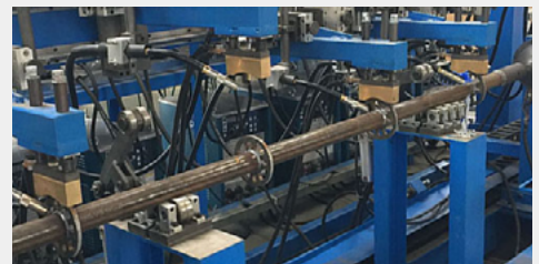
Standard and ring plate welding
