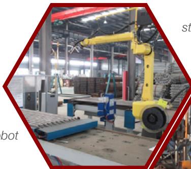
Ringlock scaffolding standard welding machine
